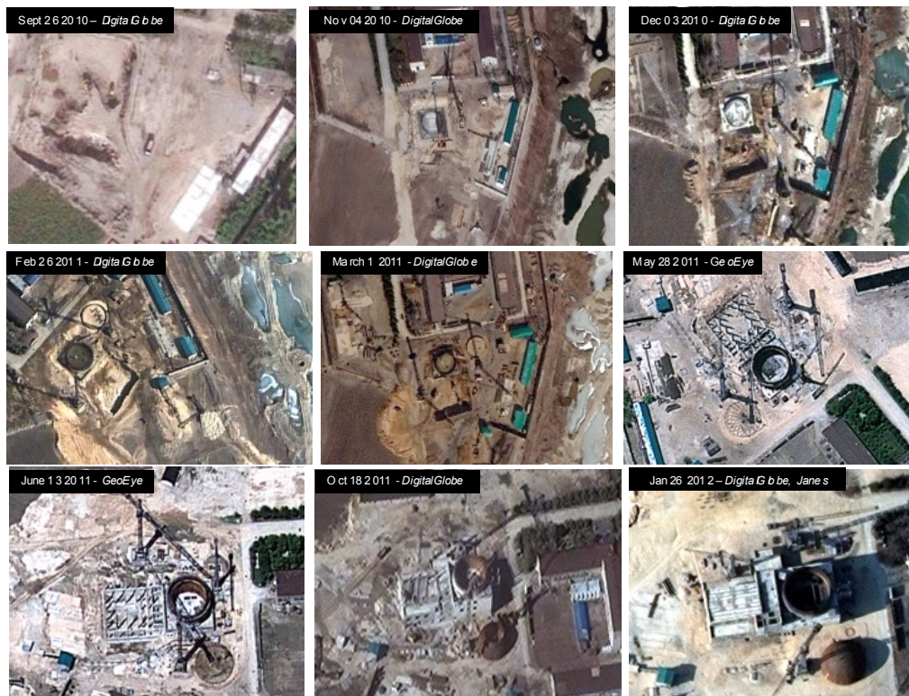
Figure 1 – A time sequence of overhead images of the light water reactor site tracking its development from September 2010 to November 2011
