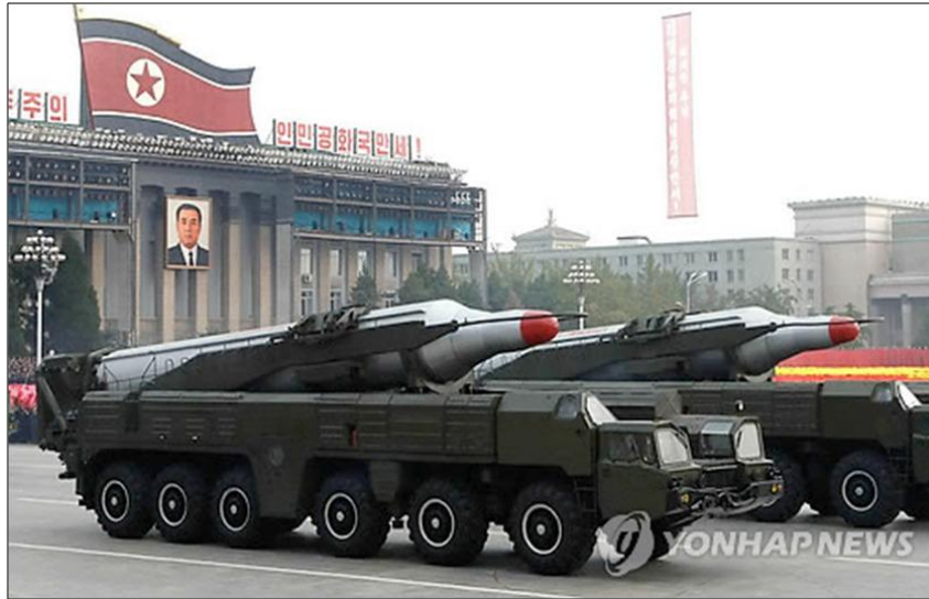
Figure 8 – Side View of the Musudan IRBM missile and MAZ-547A TEL as featured in the 10 Oct 2010 military parade in Pyongyang. Source: (KCNA-Yonhap News)
